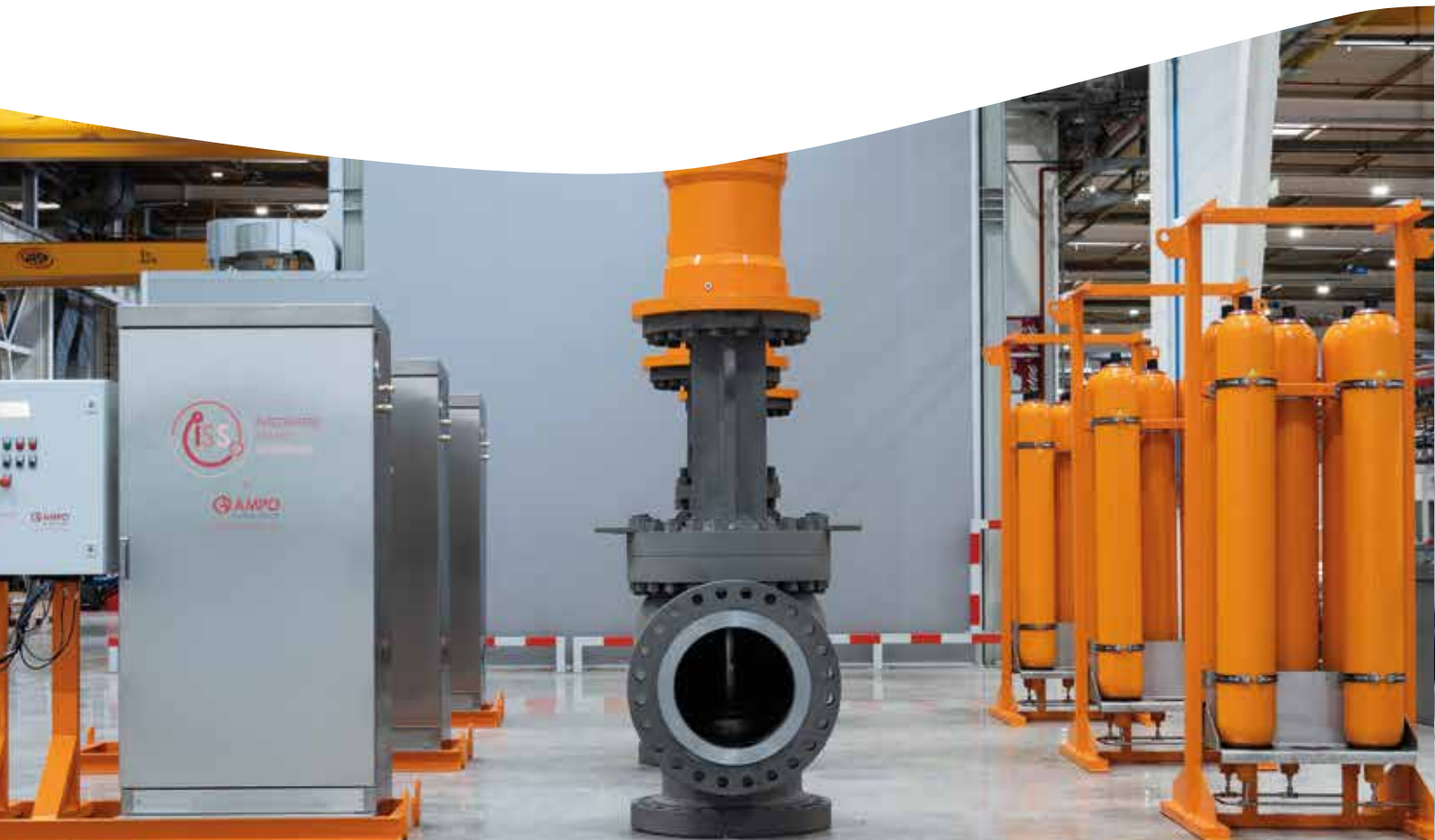
Emergency shutdown integrated system
