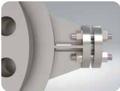
Welded standard connection mechanically reinforced connection to avoid load transmission to welding
