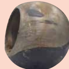
Ball after 1000 cycles. Wear appears in the ball, removing the coating.
