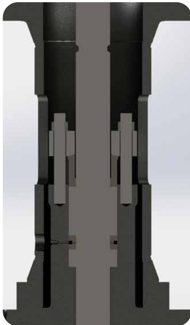
Double Barrier Graphite Packing separated by metal ring
