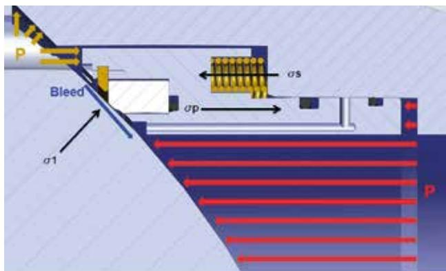
Double Isolation Bleed valves are also available where single valve with two seating surfaces is supplied, each of which, in the closed position, provides a seal against pressure from a single source, with a means of venting/bleeding the cavity between the seating surfaces. This feature can be provided in one direction or in both directions (SPE/DPE or DPE/DPE with an external bleeding system).
