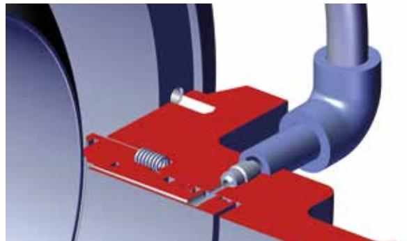
An emergency sealant injection system through the seat up to the ball and through the stem are available for restoring stem and/or seat tightness in case of damages of sealing components (O-ring or seat inserts) due to the presence of solid particles in the process fluid.
